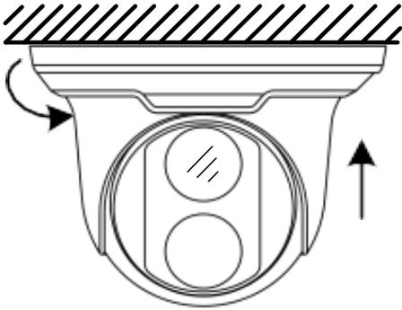
Push the bottom ring back up and turn it clockwise to lock into position
