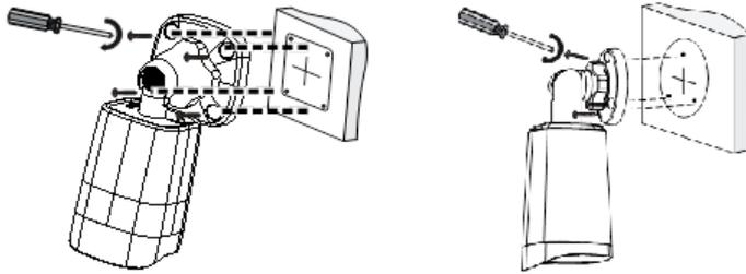
Lead tapping screws through the guide holes in the base and fix them on the wall by using a screwdriver.
