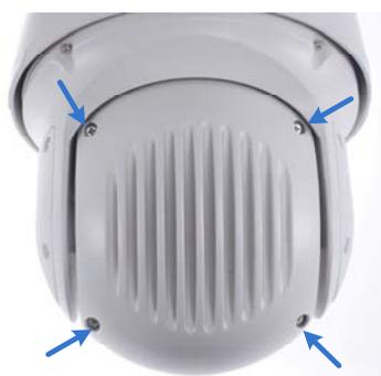
2. Insert the micro SD card into the slot, and secure the back cover of the camera.
