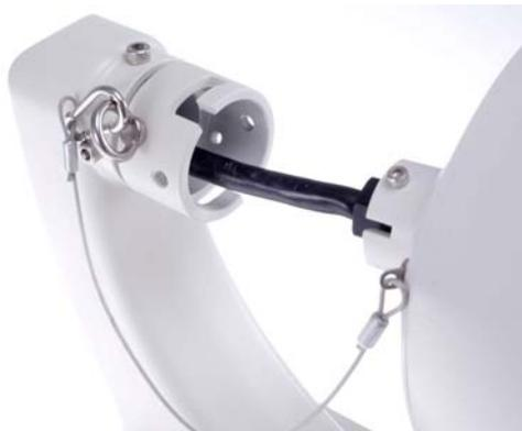
7. Attach the camera to the pendant tube, rotate the camera until it is locked into position, and secure the indicated screws.
