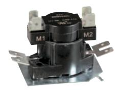
The positive temperature coefficient (PTC) heater element provides voltage compression over a wide voltage range without danger of over-heating at high voltage. It is self-current limiting, and assures device actuation under low-voltage conditions. The PTC has the unique feature of always stabilizing at a specific temperature, regardless of ambient temperature or voltage. This will allow the use of a common device over a wide voltage range.
