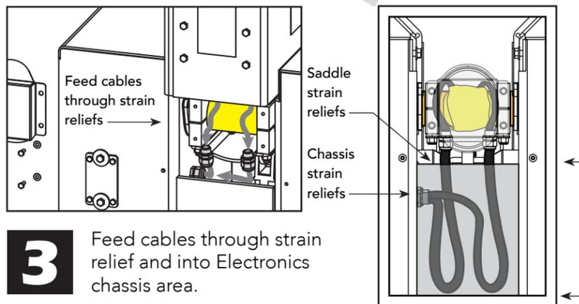
**3** Feed cables through strain relief and into Electronics chassis area.
