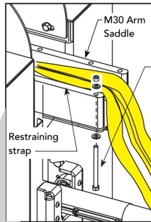
**2** To stabilize the bottom clamp, return one fastener to the front edge of the saddle. Keep the nut loose while installing the straps and aligning the upper catch pin.
