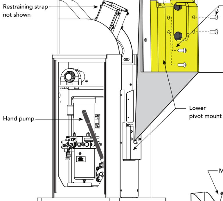
Loosen and remove the four button head screws from the bearings prior to installing the lower arm.
