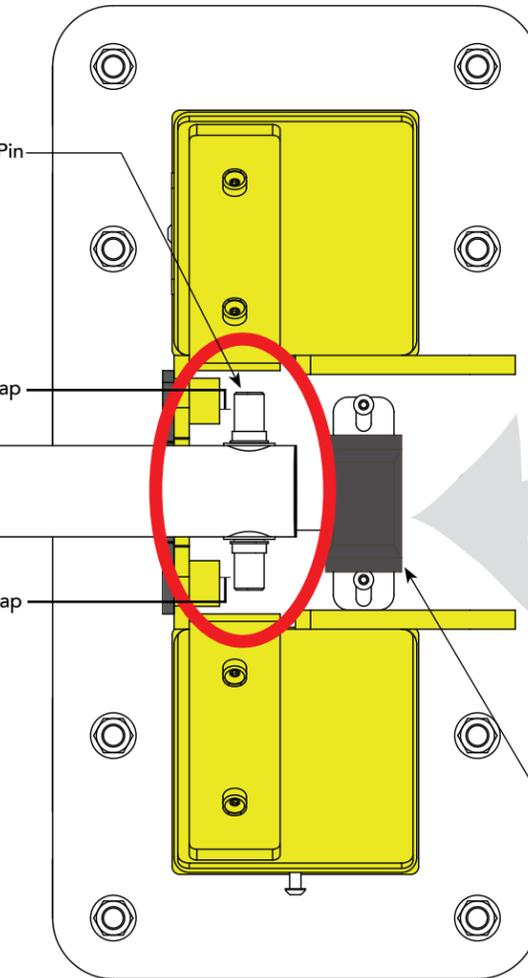
**5** With the gap clearance set at approximately 3/4-inches between the Lower Catch Pin and Post, securely tighten the top clamp (see step 3) on the Lower Pivot Assembly.
