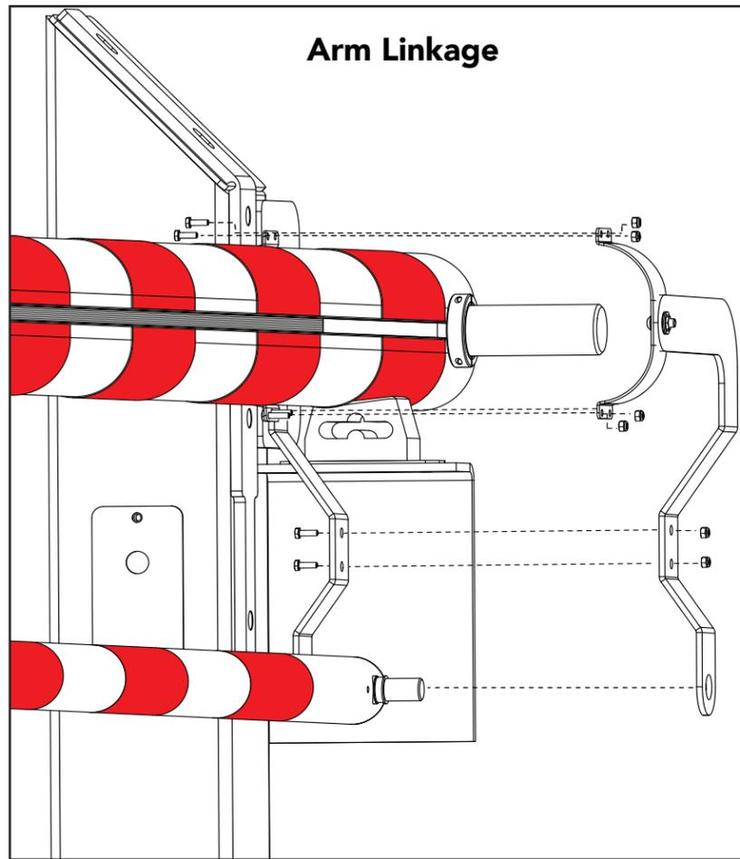
**4** Assemble the Arm Linkage as shown in the illustration. Tighten the fasteners securely.
