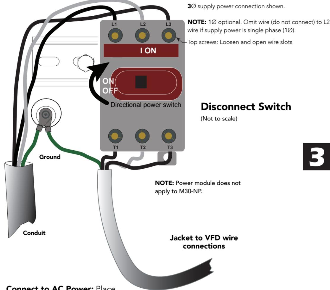
**2 Connect to AC Power:** Place the incoming power wires into their appropriate slots. Attach the ground wires to the chassis.
