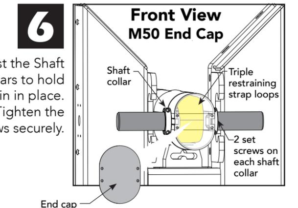
**6** Adjust the Shaft Collars to hold the pin in place. Tighten the 4 screws securely.
