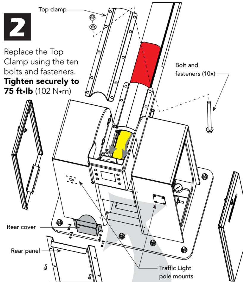
**2** Replace the Top Clamp using the ten bolts and fasteners. **Tighten securely to 75 ft·lb (102 N·m)**
