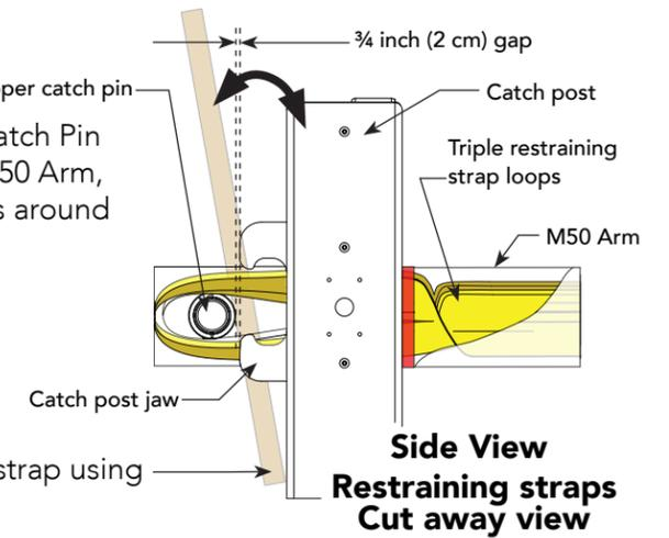
**4** To support its weight, rest the M50 Arm on the Catch Post's bumper. Ask for assistance and feed the pivot pin through the restraining straps.
