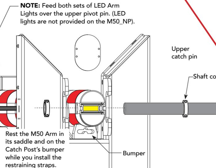
**7** Position the End Cap and secure it using four hex head screws (provided).
