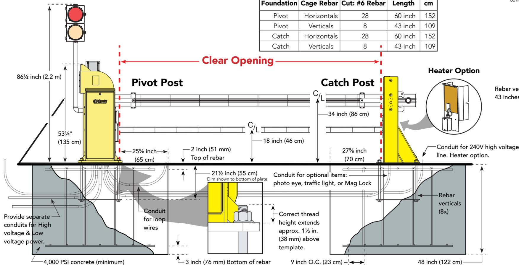
**4** Install the anchor bolt assemblies as shown.
