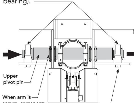
When arm is secure, center arm in saddle. Make slight adjustments, using a 7/16-inch socket wrench. Loosen 2 nuts on interior flange.
