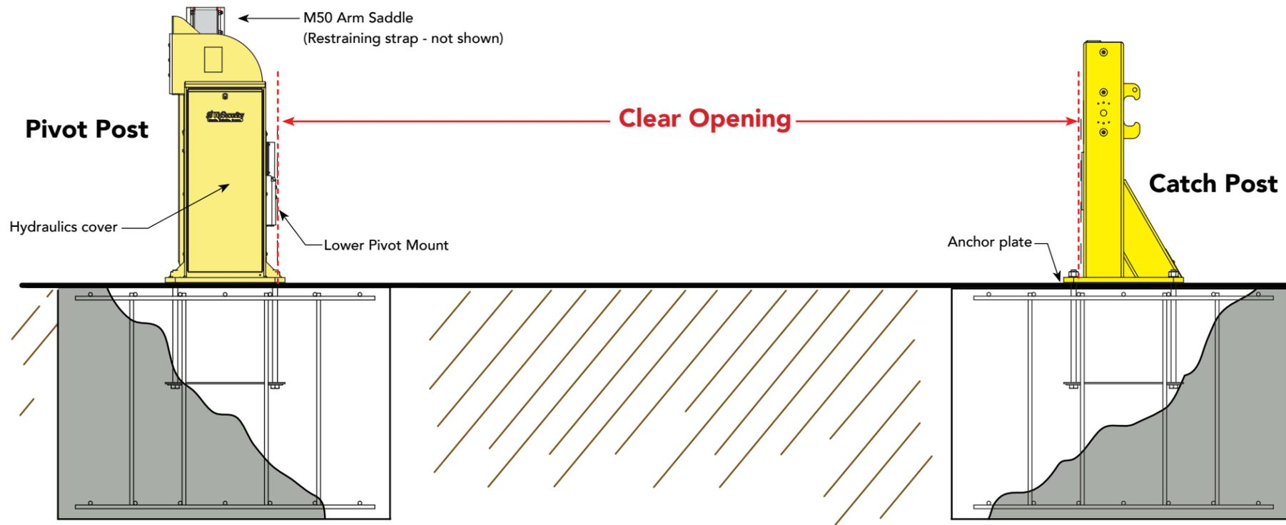
**3** Ensure the posts are plumb. Shim or grout as required.
