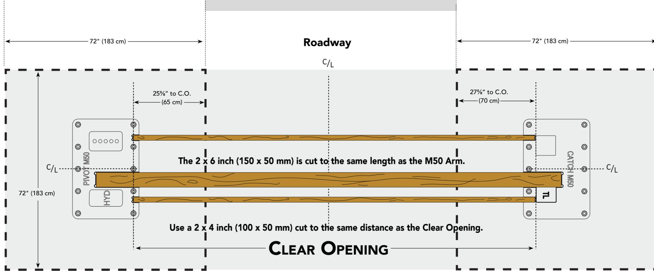
**2 Measure and mark the excavation pit.** Mark the conduit openings and locate the conduit trenches and rebar cages accordingly.
