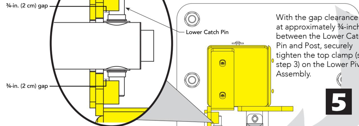
With the gap clearance set at approximately 3/4-inches between the Lower Catch Pin and Post, securely tighten the top clamp (see step 3) on the Lower Pivot Assembly.
