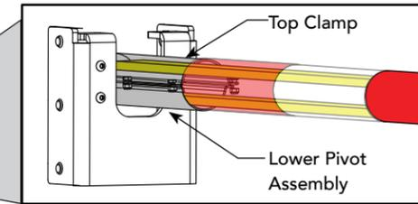
**4** Slide the Lower Arm to obtain 3/4-inch clearance at the Catch Post.
