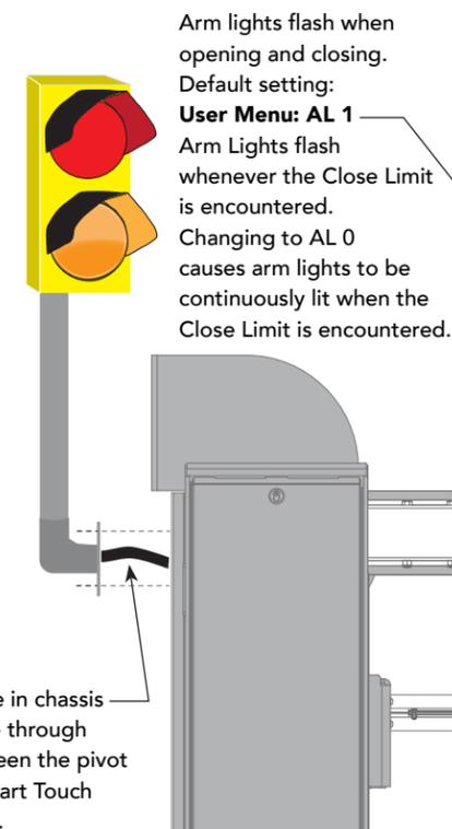
Feed wire through hole in chassis and, if necessary, route through supplied conduit between the pivot posts to access the Smart Touch Controller connections.
