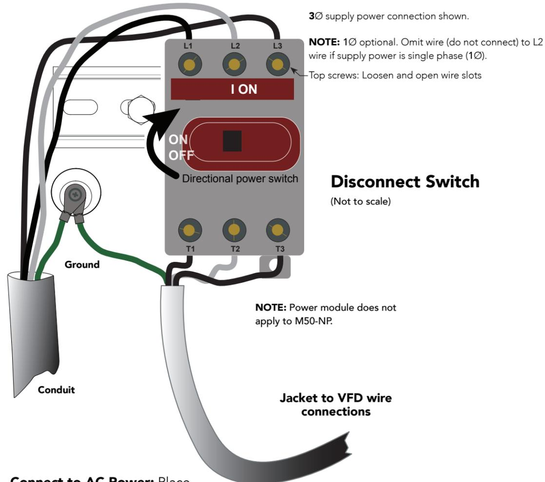
**2 Connect to AC Power:** Place the incoming power wires into their appropriate slots. Attach the ground wires to the chassis.
