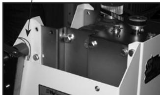
**4** Remove the drive belt. Use a ⅝-inch socket wrench to loosen (do NOT remove) the 4 bolts securing the motor to the motor plate.
