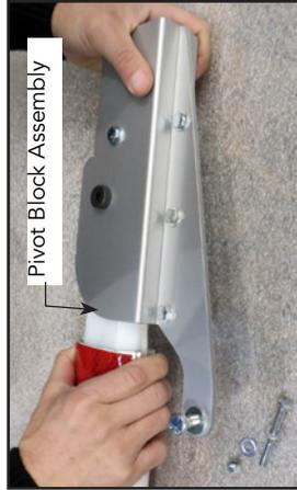
**3** Secure Pivot Block with supplied fasteners. Use box-end and socket wrenches. Tighten bolt securely.
