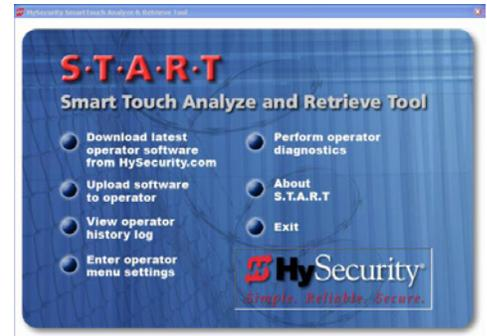
With S.T.A.R.T. software loaded on your laptop computer, you have an invaluable management tool for all HySecurity operators. The USB port, allows you to download system diagnostics and upload system configurations using the S.T.A.R.T. software. The free S.T.A.R.T. software is conveniently located at [www.hysecurity.com](http://www.hysecurity.com). Instructions for downloading S.T.A.R.T. are on the website.
