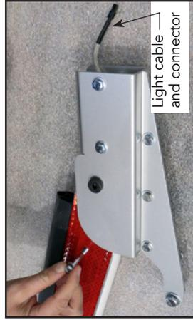
**6** Insert Pivot Block Assembly into aluminum arm. Guide light cable through Pivot Block hole. Create a cable loop. See CAUTION.
