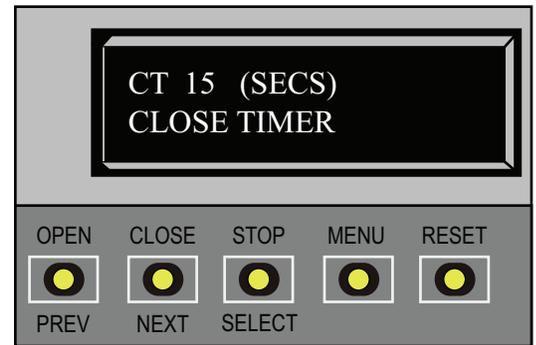
The Close Timer assigns how many seconds will pass before the operator initiates closure of a fully opened barrier arm after all open commands and reversing sensor inputs have ceased and loops cleared. Every gate operator needs to have the close timer set to a specific number of seconds (for example, 5 seconds) unless a hard-wired closing device is connected to the unit, such as a “hold to close” push button station.
