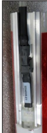
**2** Insert Pivot Block Assembly into aluminum arm. Guide light cable through Pivot Block hole.
