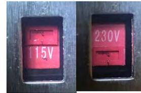
Figure 27. Voltage Switch Positions
