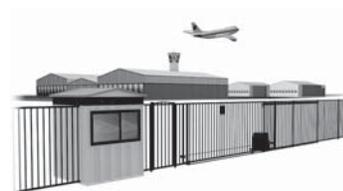
Class IV: Intended for use in guarded industrial locations or buildings such as an airport security area or other restricted access location, not servicing the general public, in which access is monitored by security personnel or via closed circuitry.
