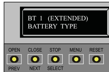
4. Use NEXT to navigate to the menu display. Change the setting using the SELECT and NEXT buttons.
