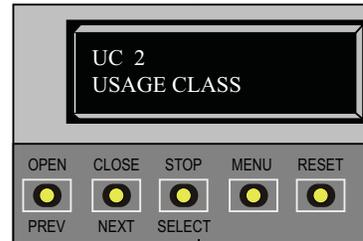
3. Access the Installer Menu, by simultaneously pressing OPEN and RESET. Release the buttons.
