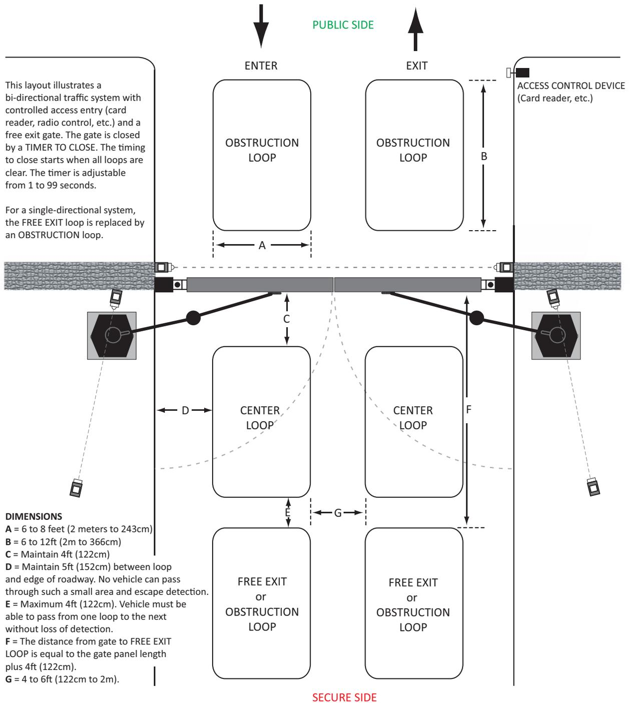
Vehicle Detectors and Loop Layout for Openings greater than 28 feet\*
