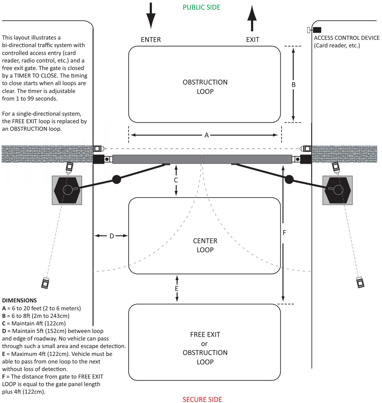
Vehicle Detectors and Loop Layout for Openings less than 28 feet\*
