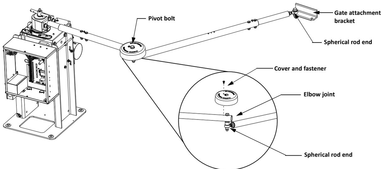
When installing an articulating arm assembly, be sure to take into account the following guidelines:
