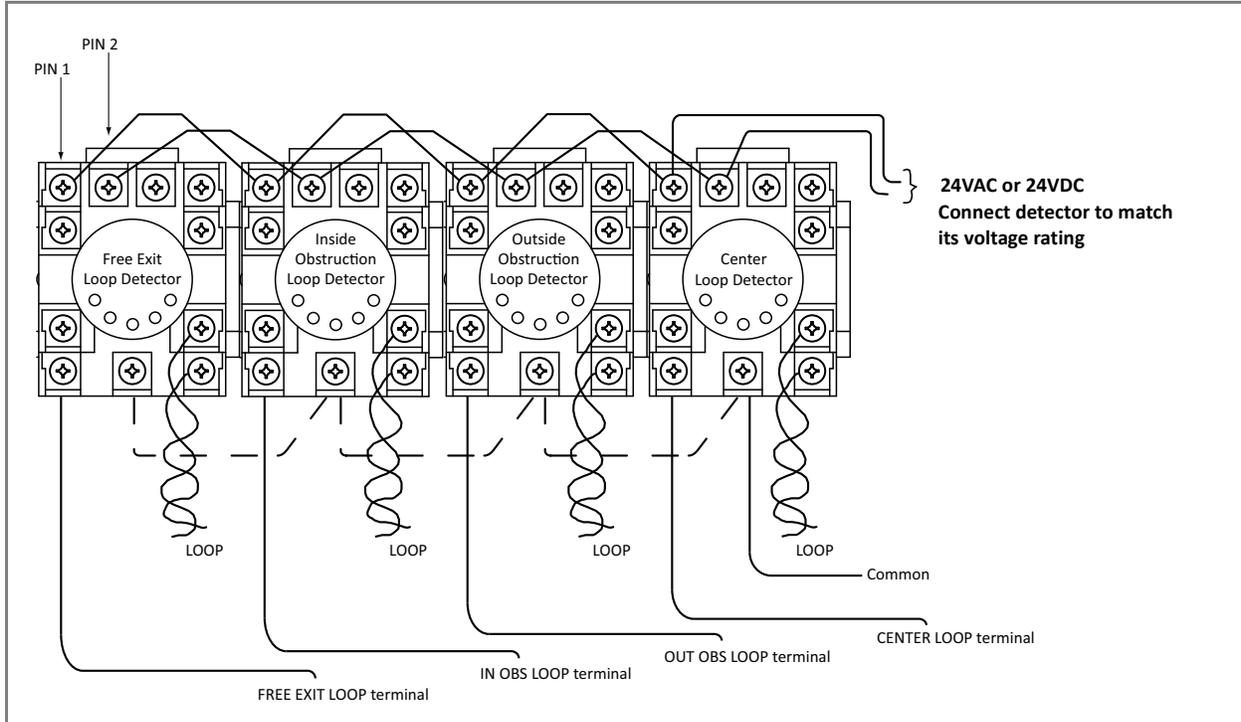
**Figure 4-4. Standard 11-Pin Box Type Vehicle Detector**
