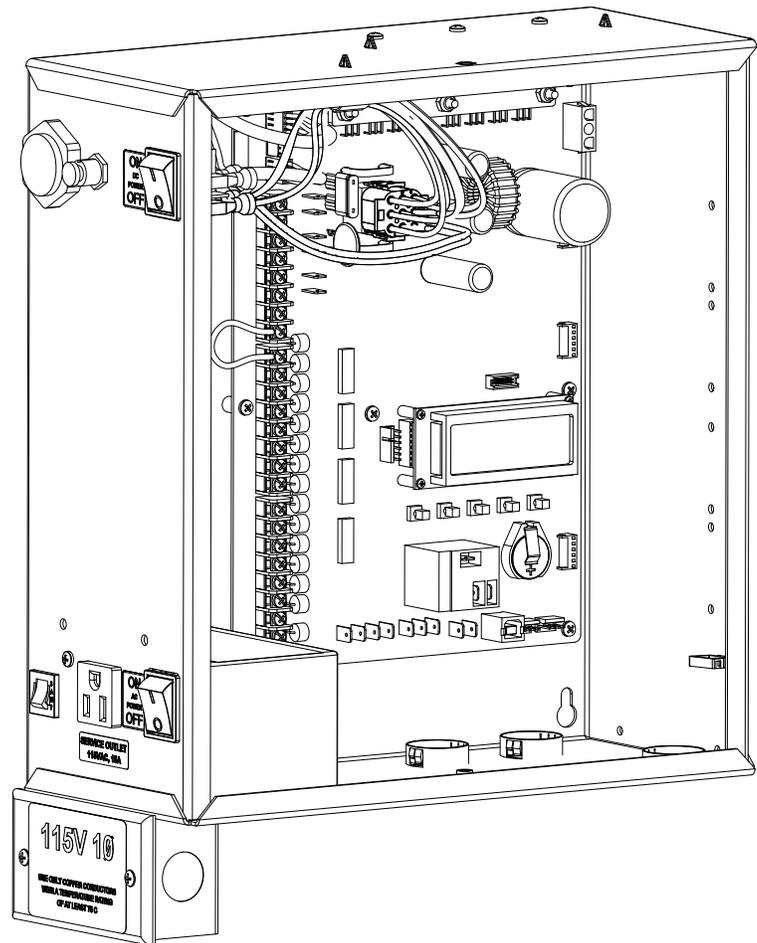
Figure 4-1. Smart DC Controller and Control Box
