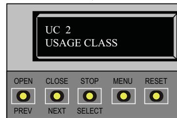
Release the buttons and the Usage Class display appears indicating entrance to the Installer Menu. The USAGE CLASS display is the first item in the Installer Menu.
