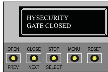
1. S.T.A.R.T. at a gate status display. To bypass the Operator Status Displays, press the MENU button twice.
