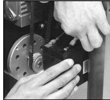
Reconnect the wires onto the replacement batteries.
