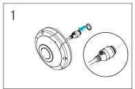
Insert a round rubber ring (silicone rubber) into the RJ45 jack.
