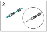
Insert the network cable into the waterproof cap, rubber bushing, and waterproof cap body in order.
