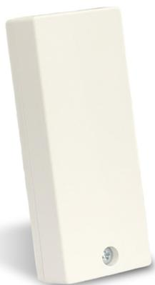
The Inovonics door/window with wall tamper and EOL has a built-in magnetic reed switch on the side with a magnet that supports a 5/8" gap. A 2.2K ohm end of line resistor is included, and is required to operate it. The transmitter includes a wall tamper switch that notifies the system when the transmitter is removed from its mounted surface.
