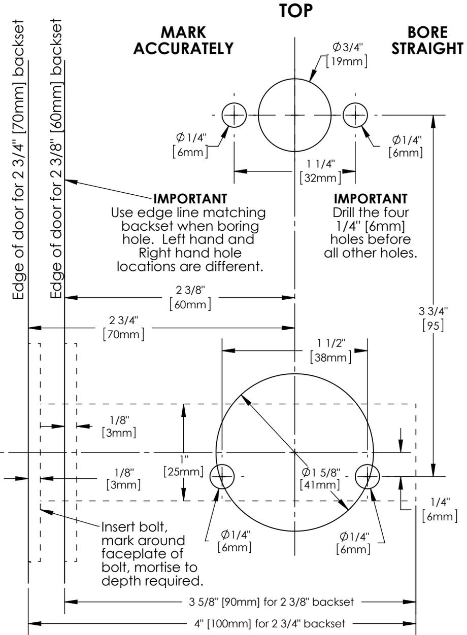
Right Hand installation for both 2 3/8" (60mm) and 2 3/4" (70mm) backsets
