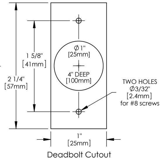
Left Hand installation for both 2 3/8" (60mm) and 2 3/4" (70mm) backsets
