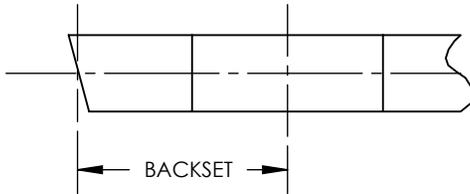
**NOTE:** Lock will accommodate doors 1 3/8" [35mm] to 2 1/4" [57mm] thick. Suitable reinforcement shall be provided by the hollow metal door manufacturer to prevent collapsing of door. When door silencers are to be installed, proper allowances must be made for strike location.
