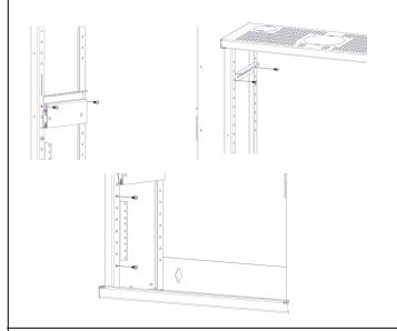
Step 4: Use a screwdriver to remove button head screws. Move the rail to the desired location. Use screw driver to fasten rail into place.
