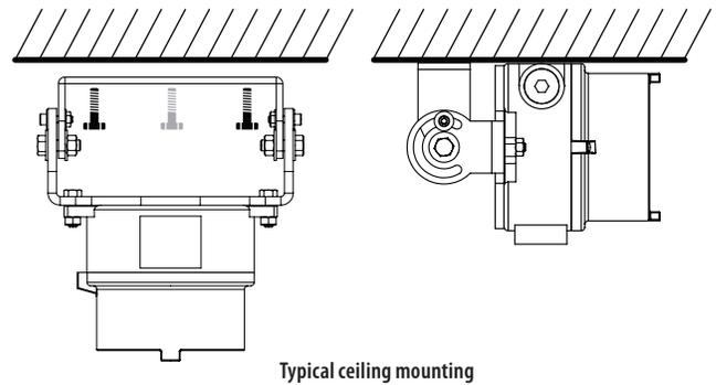
1. Mark the location of the screws that anchor the mounting base to the mounting surface. See the note above. If you are routing the drop cable through mounting surface, also mark the position of the hole for the drop cable.
