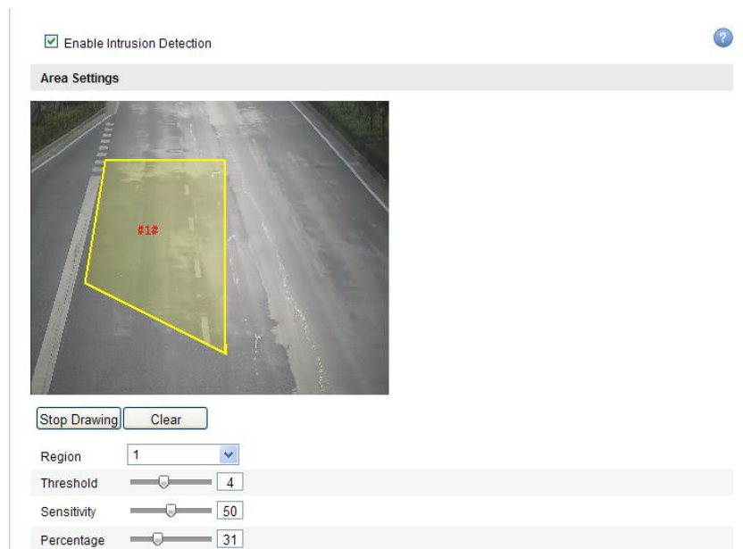
Figure 6-63 Configuring Intrusion Area
