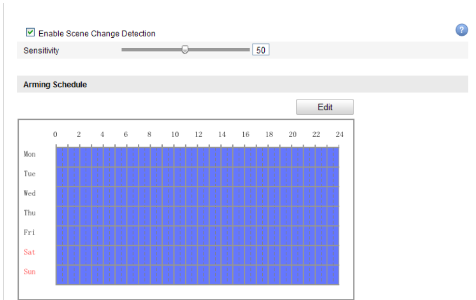
Figure 6-60 Configuring Scene Change Detection
