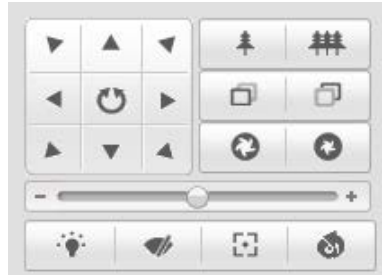
Figure 5-3 PTZ Control Panel
