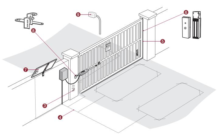
LiftMaster gate operators comply with UL 325 standards. Important: To be compliant with UL 325 and industry safety guidelines, qualified monitored external entrapment protection devices such as photoelectric sensors or edge sensors are required to be installed with this operator.
