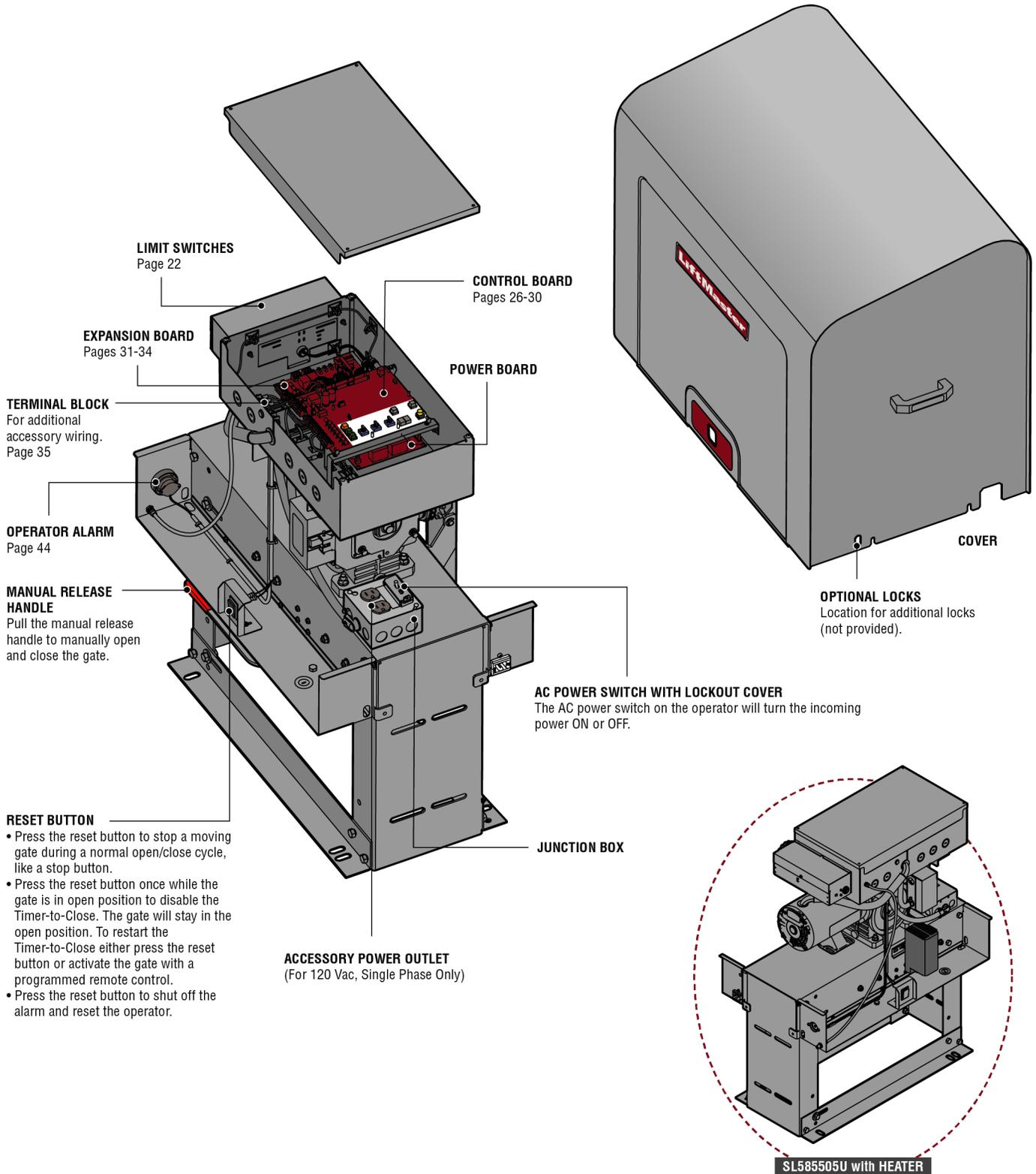
**NOTE:** The heater can only be turned off from the thermostat next to the heater.
