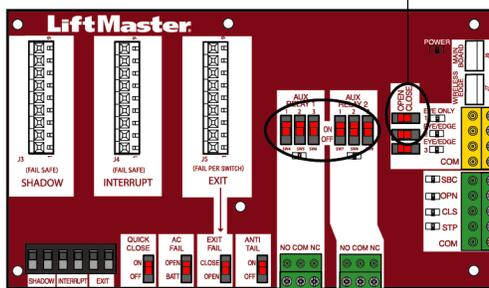
**NOTE:** These switches determine if the corresponding photoelectric sensor or edge sensor will function for the OPEN or CLOSE cycle.
