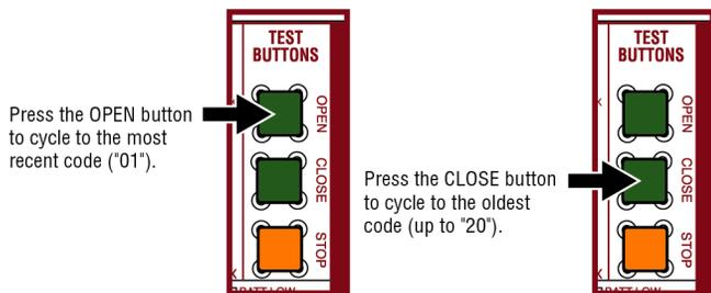
The operator will only keep track of up to 20 codes, then will start saving over the oldest codes as new codes occur.
