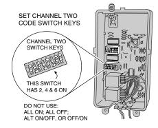
STEP 3 Transmitter code setting. Locate the coding switch on the transmitter and set the eight keys identical to those on the desired channel of the receiver. Be sure they match exactly. If using a two or four-channel transmitter, refer to the coding instructions included with the transmitter for proper system codina.
