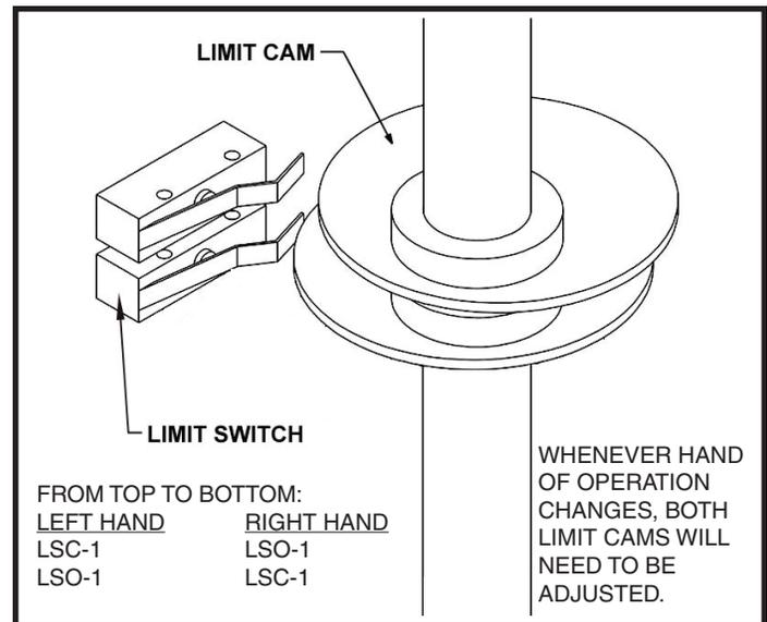
Figure 10. Model SWG Limit Switches & Cams
