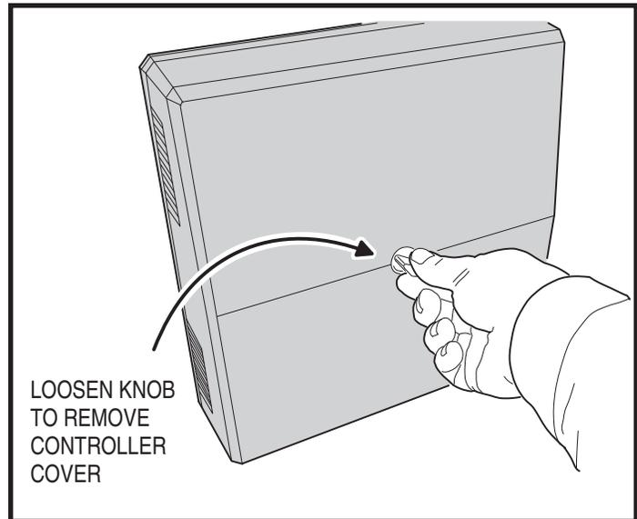
Figure 8. Controller Access
