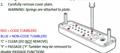
PRESS & HOLD 'C' BUTTON to release tumblers. IMPORTANT: 'C' Button must be pressed and held down when removing and inserting tumblers. Failure to do so will damage the lock and void the warranty.
