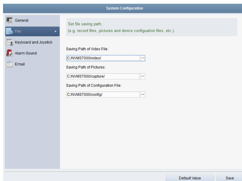
Click **Tool-> System Configuration-> File**; configure the corresponding saving path of pictures and video files. Select the window in the live view interface and press the button on the right side of the joystick to capture or press the button on the left side to record. The pictures and videos will be saved to the configured saving path.
