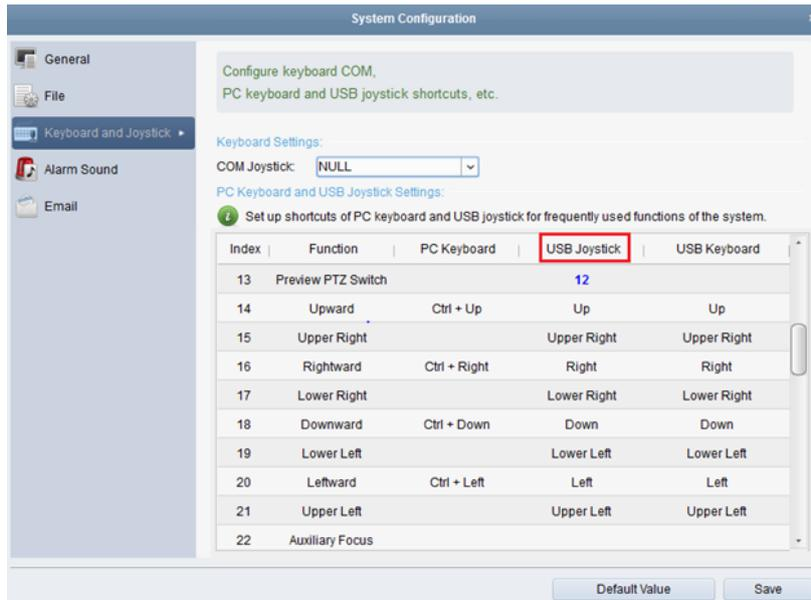
Click the **Tool-> System Configuration-> Keyboard and Joystick-> USB Joystick** on client and then configure the corresponding shortcut keys of number **1~12**. Select the window in live view mode interface and operate according to each shortcut.
