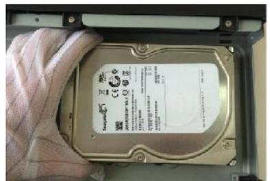
3. Put the HDD into the Device.
