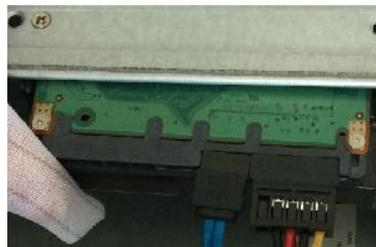
5. Use the power cable to connect HDD and mainboard.
