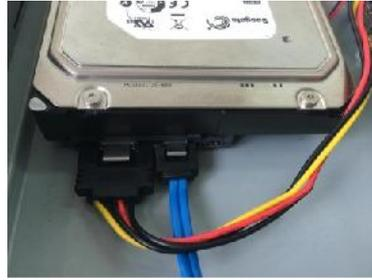
5. Use the HDD cable and power cable to connect HDD and mainboard.
