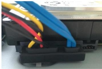
5. Use the HDD cable and power cable to connect HDD and mainboard.
