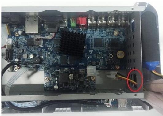
1. Pull the battery cable through the hole.
