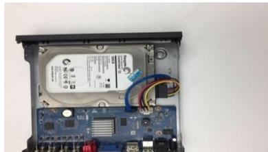
5. Connect the HDD cable and the power cable to the mainboard.
