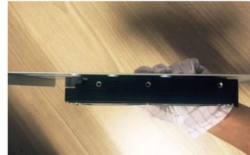
3. Put the HDD onto the bracket.
