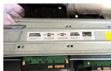
2. Fix the HDD(s) onto the bracket. Remove the top bracket if you want to
