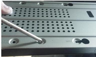
5. Use screws to fix the HDD onto the bracket.
