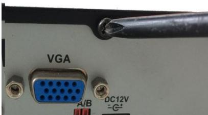
1. Remove the screws on the rear panel.
