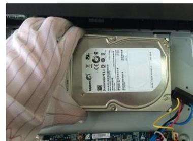
3. Place the HDD onto the Device.
