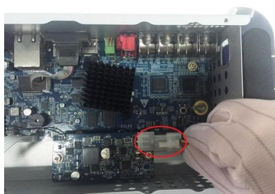
2. Connect to the cable into the port.
