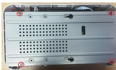
8. Install the bracket back and then fasten the screws.
