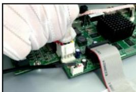
Figure 2-3 Connect Power Cable
