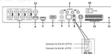
Figure 2-5 Controller Connection A
