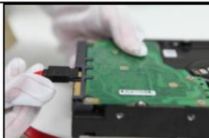
Step 4 Place the HDD on the bottom of the device and then fasten the screws on the bottom to fix the HDD.
