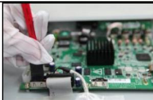
Figure 2-2 Connect Data Cable
