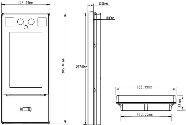
A waterproof hood is required in waterproof installation. The figure below shows the dimensions of the waterproof hood.
