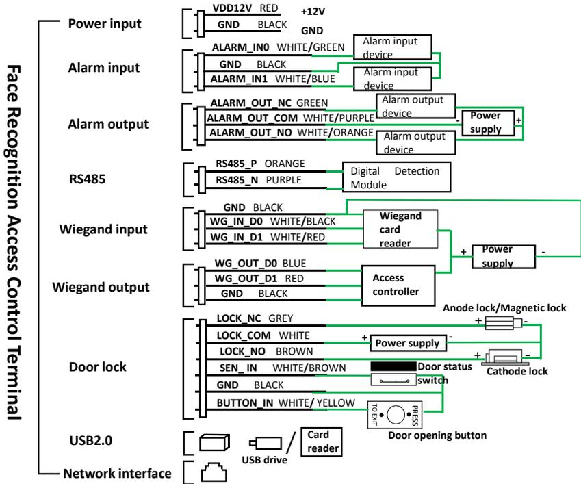
The face recognition access control terminal can be also connected to a security module. The figure below shows the wiring of the security module.
