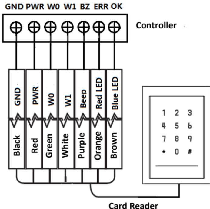
Figure 2-5 Wiring for Wiegand Communication Mode
