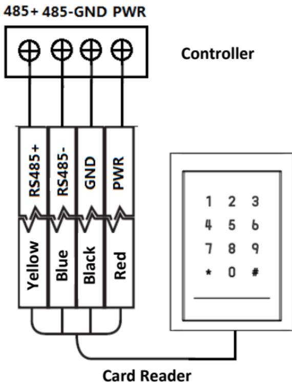
Figure 2-4 Wiring for RS-485 Communication Mode
