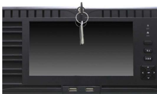
Figure 2. 2 Insert Panel Key
