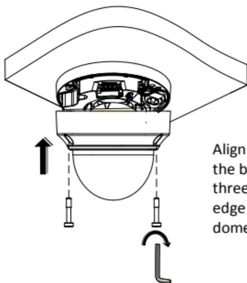
Align the screw holes in the base and tighten the three torx screws on the edge of the transparent dome cover to fix it
