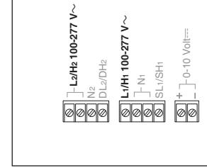
Class 2/PELV, 0-10 V--- wiring from a ballast/driver to the GRX-TVI must be separated from the power wiring. Enter the Class 2/PELV wires through the knockout adjacent to the 0-10 V--- terminal blocks. The barrier ensures separation and is flexible to allow access to the terminals. The barrier must be in place when installation is complete.
