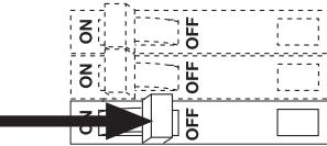
**Note:** Multiple power feeds could be provided. Ensure that all feeds are off before wiring.
