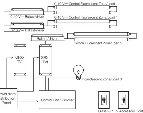
**Note:** When using a Control Unit, a GRX-TVI is required for each 0-10 V--- fluorescent zone. (A 3-zone Control Unit with two fluorescent zones and one incandescent zone is shown as an example.)
