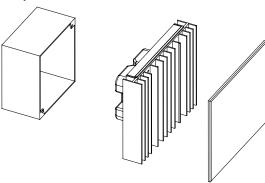
Mount to 4 × 4 in (102 × 102 mm), 2.1 in (53 mm) deep U.S. junction box with barrier (for 277  $V\sim$  loads if required by local electrical code)
