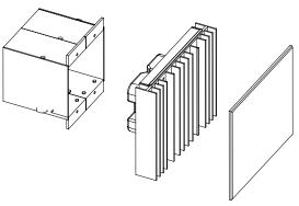
Mount to  $4 \times 4$  in (102 × 102 mm), 2.1 in (53 mm) deep U.S. junction box
