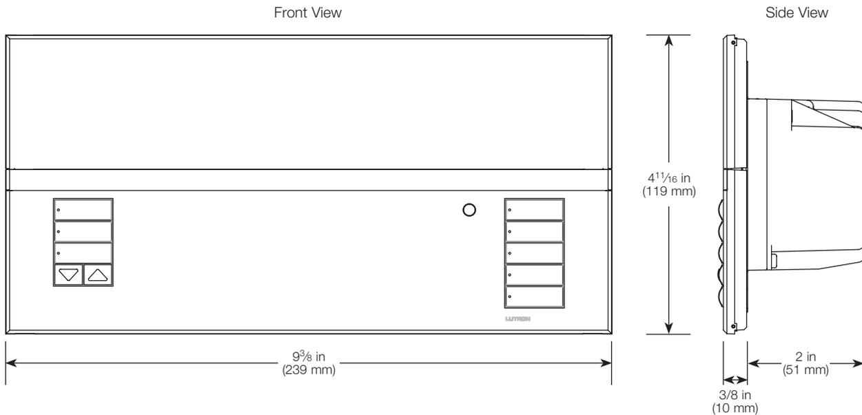
Fits into a 4-gang U.S. backbox, 3 1/2 in (90.4 mm) deep (Lutron P/N 245254) or 3 in (76.2 mm) deep (Lutron P/N 241400)
