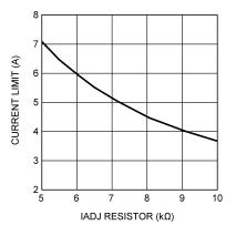
Figure 7-3. Current Limit vs IADJ Resistor
