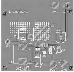
Figure 10-2. LM22679 Layout Example
