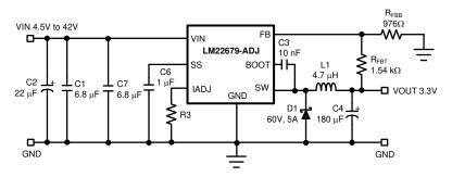
Figure 8-2. Typical Buck Regulator Application
