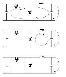
Figure 10-1. Current Flow in a Buck Application
