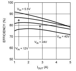
Figure 8-3. Efficiency vs I<sub>OUT</sub> and V<sub>IN</sub> (V<sub>OUT</sub> = 3.3 V)
