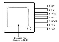
Figure 5-1. 7-Pin NDR Package Top View
