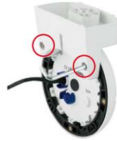
4. Use the Torx screw to fasten the mount onto the wall. Make sure that the head of the screw is not tight against the wall, but that it still has 5 mm/0.2 in to go.
