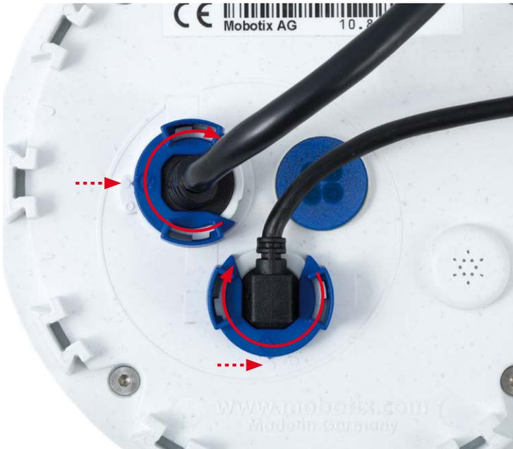
Close the cable retainer by rotating the bayonet catch to the marked position
