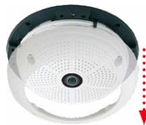
2. **Remove the camera mounting ring:** Separate the black mounting ring from the camera housing. This ring is not required when mounting the camera to the Wall Mount.
