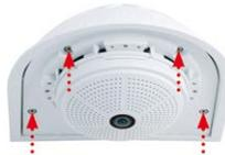
9. **Attach the outer shell:** Position the outer shell (without the rubber seal) and tighten all four Allen screws using the included Allen wrench.
