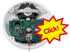
2. **Mount the back plate:** Replace the back plate of the camera housing, ensuring that the back plate screw holes are correctly positioned above the thread inserts.
