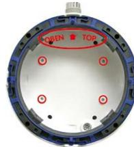
4. **Cable feeding:** Attach the counternut to the network cable, pass it through the seal from the outside and tighten the nut. The network cable is now screwed into the On-Wall Set, weatherproof. All unused openings must be sealed with the included sealant plugs. The cable passing into the housing must always be installed using the supplied three-part fittings.
