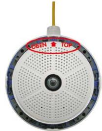
9. **Attach the outer shell:** Position the outer shell without the rubber seal and tighten all four Allen screws using the included Allen wrench.
