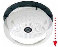
4. **Remove the mounting ring:** Separate the mounting ring from the camera housing. This ring is not required when mounting the camera in the In-Ceiling Set.
