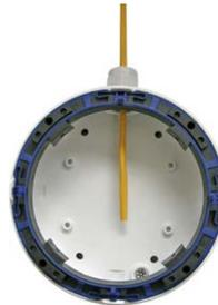
5. **Remove the camera outer shell:** Unscrew all four Allen screws with the supplied Allen wrench. Remove the outer shell.
