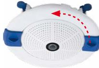
Removing the decorative ring: turn counter-clockwise - only relevant when completely removing the camera
