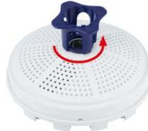
3. **Replace the lens:** Screw the lens back in using the lens wrench.
