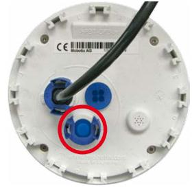
2. **Remove bayonet catch and USB plug:** Turn the bayonet catch to the left (red arrow in figure), take it off and remove the blue USB plug.
