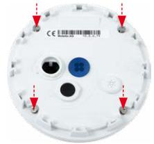
3. **Screw the back plate tight and replace the connection cables:** Place the four Allen screws back into the back plate and tighten the screws using the supplied 2 mm Allen wrench. The previously removed patch cable must now be reconnected (see «Attaching the Cable Retainer» in Section 2.2.2, «Procedure»).
