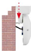
6. Properly tighten the Torx screw to secure the assembly in the desired position. There is a special hole in the Stand/Wall Mount to access the Torx screw.
