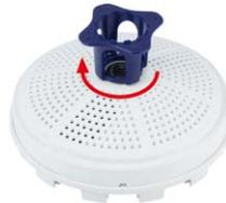
4. **Adjust the live image:** Establish a connection to the camera as described in *Section 3.1* and the following sections. The live image from the camera should be visible on the computer monitor. Select the highest available image resolution. Check image sections (image center and focus) on the computer monitor and adjust the lens with the lens wrench if necessary.
