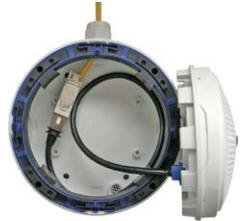
8. **Attach the camera to the mount:** The camera must be seated firmly within the On-Wall mount. The tapered guides at the back of the camera housing fit exactly into the openings of the On-Wall mount. Once, again, ensure that OBEN / TOP arrow points in the correct direction.
