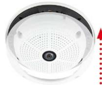
9. **Clean the lens:** If necessary, gently clean the front of the lens with a soft cotton cloth. Do not apply excessive pressure to the surface of the glass when cleaning the lens.
