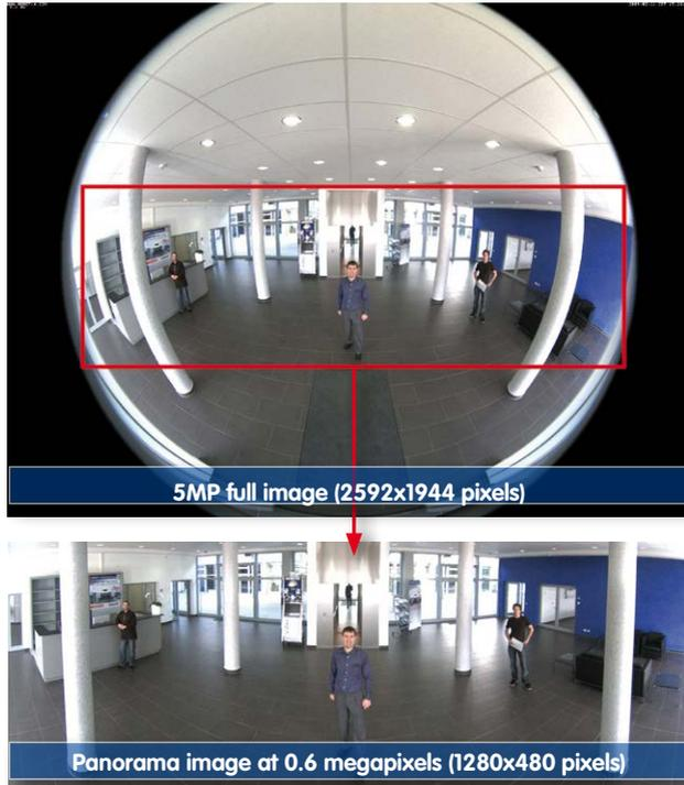
**Example:** The people marked by the red circle in the middle area of the image would not have been recorded by a regular PTZ camera; the full image recording of the Q25M allows to determine for example, the exact time at which the people entered the image area recorded by the camera. A **Browser** (Internet Explorer with MxPEG ActiveX plug-in), **MxControlCenter** or **MxEasy** can be used to examine the recorded sequences.
