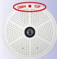
The OBEN / TOP label is only visible when the outer shell is removed
