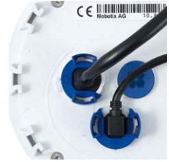
**Removing the Cable Retainer**
