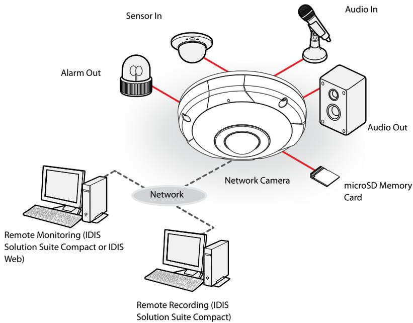
Control the camera over the network from software installed on a computer.
