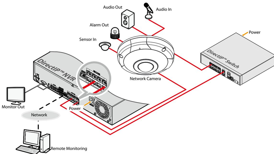
DirectIP™ NVR makes it easy to use cameras without extra network configurations. Each camera can be controlled via the DirectIP™ NVR setup menu, without any PC. For detailed camera settings, please see the camera setting pages of DirectIP™ NVR manual.
