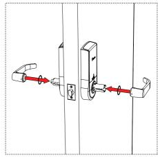
Optional step: Inserting the handle washers
