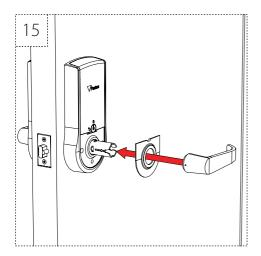
Step 12: Fitting the cover plate and handle
