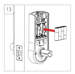
Step 10: Fitting the batteries
