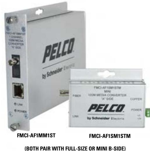
**FMCI Series** Ethernet media converters are designed to transmit and receive 10/100 Mbps data over multimode or single-mode optical fiber with ST optical connectors. The electrical interface will autonegotiate to a 10 Mbps or 100 Mbps Ethernet rate without any adjustments. The optical interface operates at a 100 Mbps Ethernet rate.
