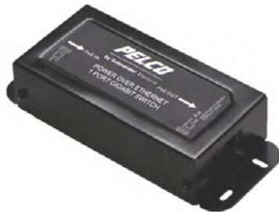
The **POE1XT** is a single-port Power over Ethernet (PoE) Gigabit extender that is designed to meet the demanding data rate and power requirements of IP cameras with high-quality streaming video capabilities. The **POE1XT** provides a voltage boost to the PoE adding another 100 meters to extend Ethernet to 200 meters (656.17 feet).
