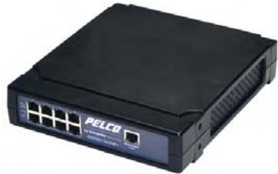
The **POE4ATN** Power over Ethernet (PoE) 4-port midspan is designed to meet the demanding data rate and power requirements of IP cameras with high-quality streaming video capabilities. The midspan offers total output power of 33.6 W per port, and meets the IEEE802.3at standard for detection, connection, disconnection, and fault protection. It also provides SNMP network management.
