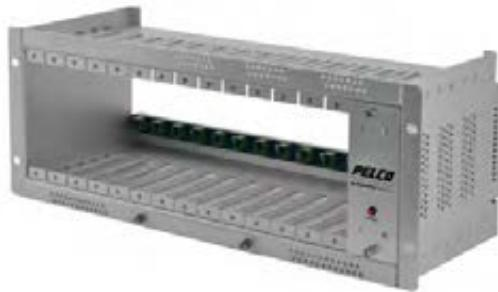
The **EURACK/USRACK** chassis is designed to hold up to 14 single-width fiber optic modules. The internal power supply is 4 RU high. The chassis is designed to mount into an EIA-standard, 48.26 cm (19-inch) rack. Optional single-width blank modules (RACK1B) can be inserted into empty module slots.
