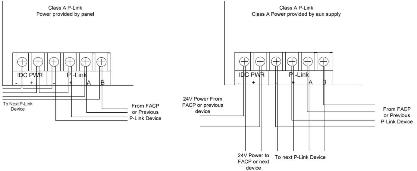
**FIGURE 5. EXAMPLE OF WIRING A IDC-6 MODULE CLASS A (LEFT) OR CLASS B (RIGHT)**
