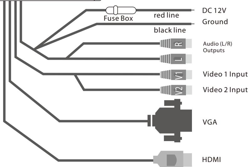
Power supply do not meet the polarity, otherwise it will damage insurance tube. (Fuse specifications: 3A or 5A)
