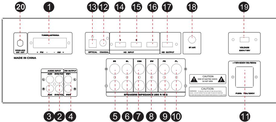
1. **TUNER ANTENNA JACK:** Properly connected AM/FM antenna
