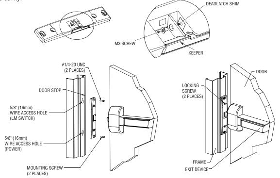
**NOTE:** Wire access hole locations are relative to the exit device orientation. **NOTE:** \*Second wire access hole required for RCI 0163LM only **NOTE:** Not to scale. Specifications are subject to change without notice.
