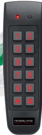
Part of the convertible line of readers/controllers, this unit can be operated as an outdoor backlit keypad reader, which connects to any standard controller, or it can convert to a fully-featured, 500-user standalone controller when connected to Rosslare's PS-x25T family of intelligent power supply/relay units. This unit provides a most effective solution for indoor and outdoor access systems where PIN credentials are required.
