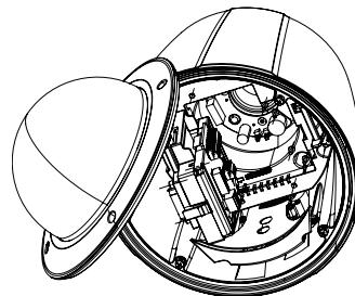
7. Please install the camera onto the housing. Please confirm that the adaptor hook is properly fixed on the camera.
