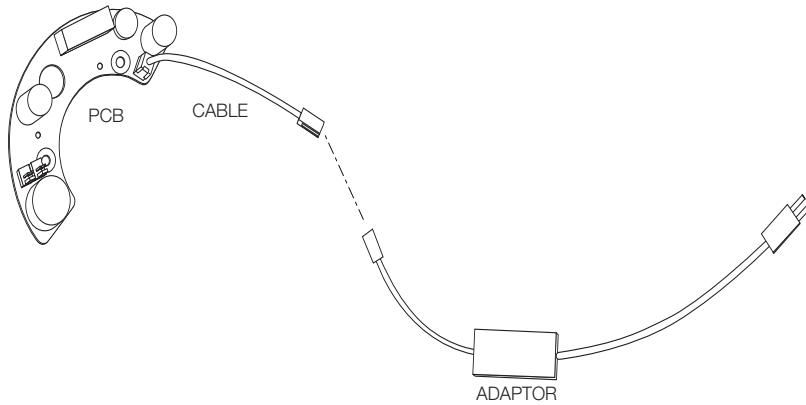
6. After inserting the external camera cable into the housing, connect it to the corresponding jack on the adaptor.
