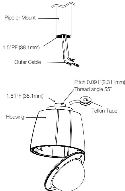
4. Install onto the pipe by turning the housing in a clockwise direction while referring to the figure below.
