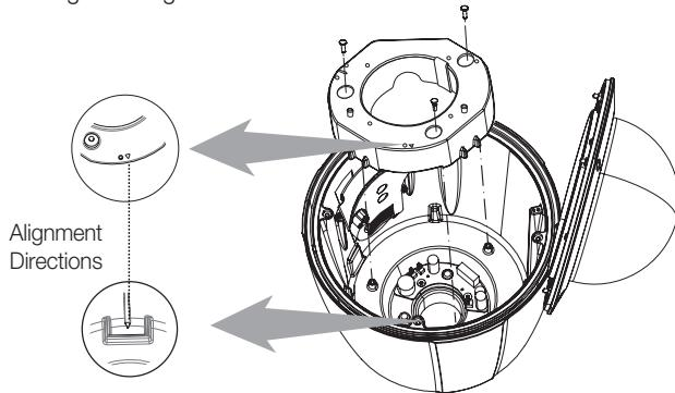
※ The lower bracket is exclusively for use with the SCP-3430 Series/SNP-5300 Series.
