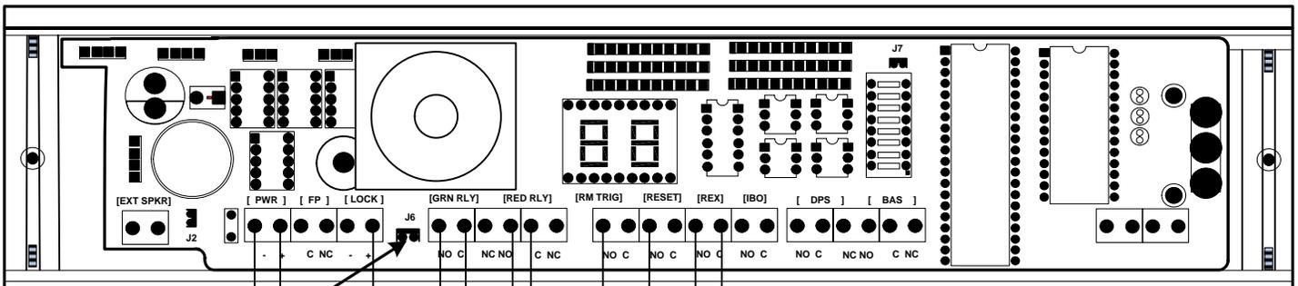
REMOVE J6 ONLY IF A FIRE PANEL OR SMOKE DETECTION SYSTEM IS CONNECTED TO [FP] INPUT (Pg. 9)
