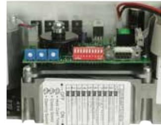
**Hold-Open Timer:** Upon receipt of an activation signal, the operator will power open the door from the closed position. The door may be held in the open position up to 30 seconds (compliance with ANSI/BHMA A156.19 requires the door to remain in the open position for a 5 second minimum). Additionally, a “hold-open” switch is provided to hold the door open for extended periods.
