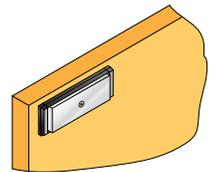
1. Align retrofit armature plate template with existing sex bolt hole.
