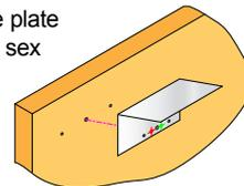
3. Attach new lock mounting plate over old mounting holes Attach 1511 or 1571 to mounting plate holes.
