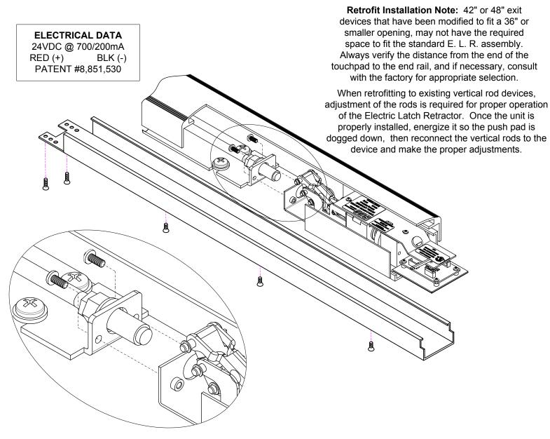
Remove the five screws from the bottom of the device (3 along the center and two on the sides attaching the head).
