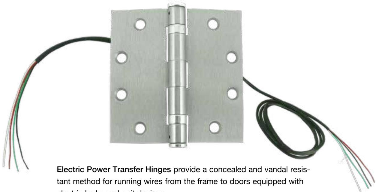
Electric Power Transfer Hinges provide a concealed and vandal resistant method for running wires from the frame to doors equipped with electric locks and exit devices.
