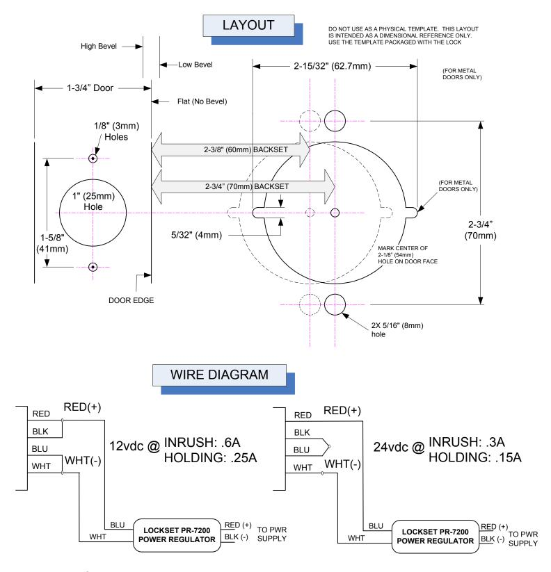
Use of the PR-7200 limits the power consumption and reduces operating temperature.
