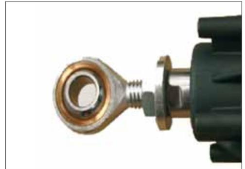
Round joint bearing for stroke adjustment
